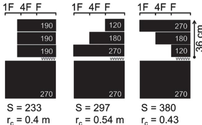
FIG. 3: EXEMPLARY SNOW STRATIGRAPHY REPRESENTED BY SLAB AND BASAL LAYERS (BLACK BARS) DISRUPTED BY A CRITICAL WEAKNESS (TRIANGLES). BELOW VALUES OF FAILURE INITIATION ( $S$ ) AND CRACK PROPAGATION ( $r_c$ ) ARE SHOWN FOR THREE LAYERINGS DIFFERING BY HAND HARDNESS (SCALE AT THE TOP), AND DENSITY (WHITE NUMBERS IN  $KG/M^3$ ). THE PROFILES HAVE THE SAME MEAN DENSITY AND HARDNESS.
